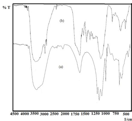
**Figure 3.** FTIR spectra of: copper (II) sulfate pentahydrate (a) and CuO nanoparticles (b)
