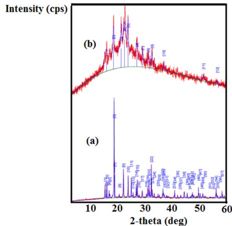
**Figure 4.** XRD powder patterns of copper (II) sulfate pentahydrate (a) and CuO nanoparticles (b).
